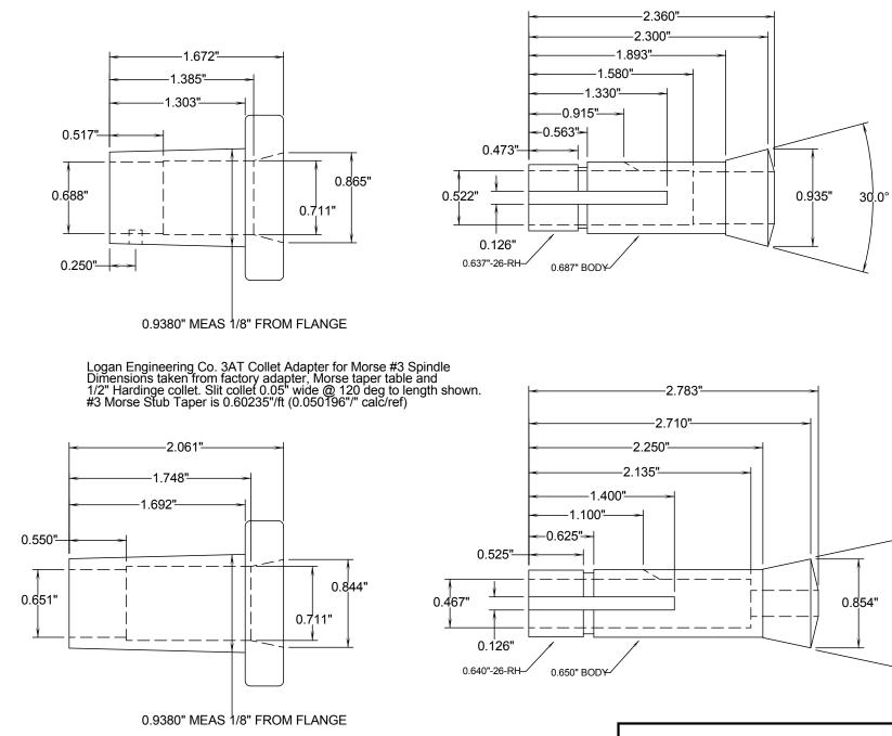
Proposed 3C Collet Adapter for Morse #3 Spindle. Check seating depth and length of drawbar! Dimensions taken from Morse taper table and 1/4" Hardinge collet. Slit collet 0.05" wide @ 120 deg to length shown. #3 Morse Stub Taper as above.
